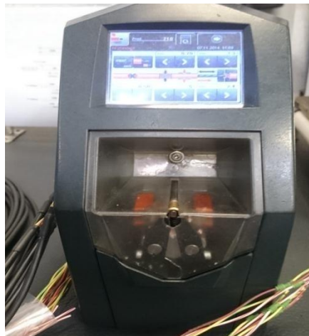
Figure 22: machine de dénudage
