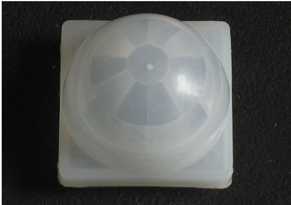
Here you can see the multiple facet-sections
