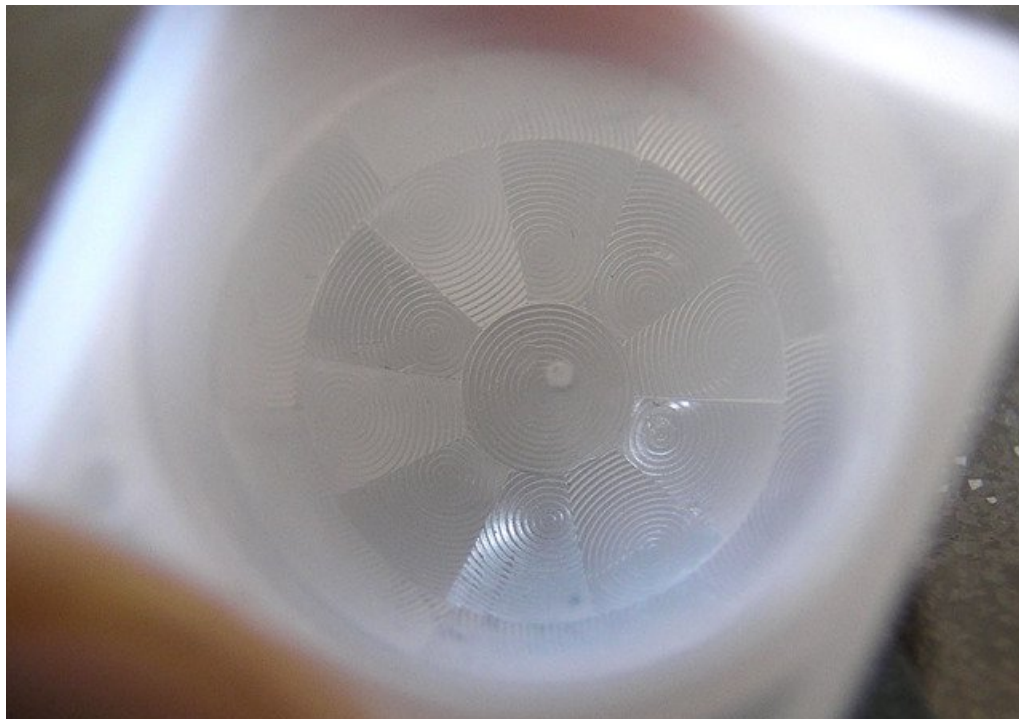
This macro shot shows the different Fresnel lenses in each facet!
